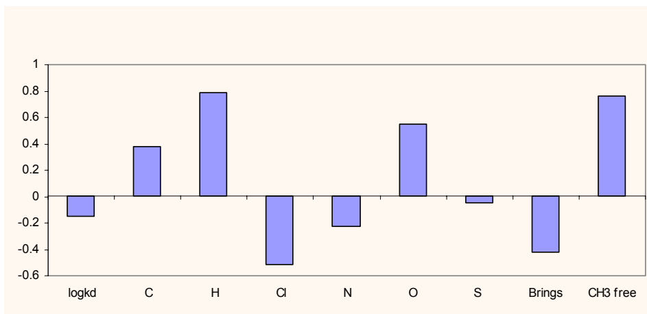
Figure 6. Correlation between water solubility of pesticides and chemical characteristics of the compounds.
