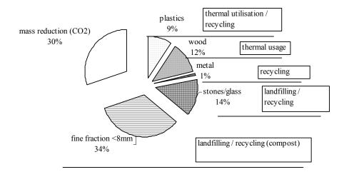
Fig. 1: Material streams and Recycling path
