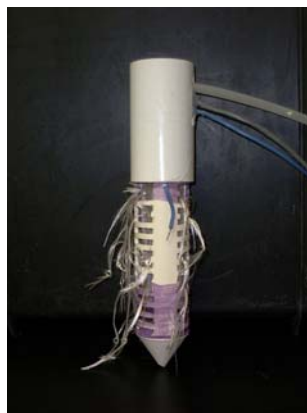
Figure 1. MTG granular moisture sensor.
