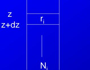
$$\boldsymbol{e} \frac{\partial y_i}{\partial t} \frac{P}{RT} = \boldsymbol{r}_{\text{DB}} r_i - \frac{\partial N_i}{\partial z}$$
