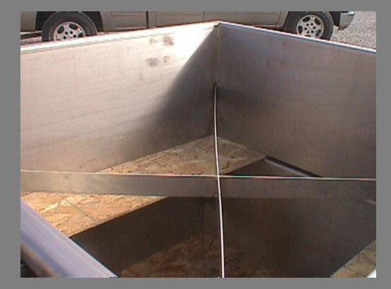
• 12 chamber collars and three chamber lids were fabricated • collars remain in ground throughout the test program
