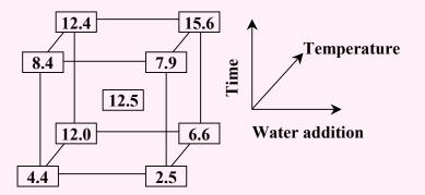
The cube plot shows the average of highest forces that can be hold by the samples (in kN). Samples with all factors set on high level had the highest mechanical strength.
